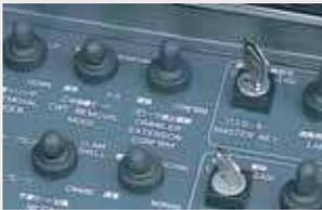
This feature prevents the crane from toppling if the boom or swing is mistakenly operated when the crawlers are being retracted. When the crawlers are in retraction mode (the load will not be displayed on the overload prevention mechanism), lowering the switch to 'confirmation' for two seconds will put it into crawler extender mode. A voice will prompt reconfirmation.
