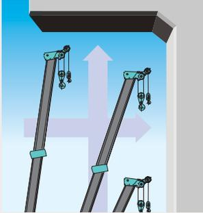
By setting the parameters of boom angle (upper and lower limits), boom top height, and operating radius, the operator can limit the range in which the boom operates. A warning buzzer sounds and the machine stops automatically whenever those limits are approached. This mechanism has proved successful on wheel cranes, and can be used not only to prevent contact, but also to increase efficiency in repetitive tasks.
